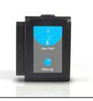
The internal humidity sensor utilizes a dielectric polymer to absorb water molecules. As more water molecules enter, the capacitance changes proportionally to the relative humidity value. Using this technique an accurate relative humidity value is calculated.
