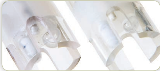
The single-junction electrode on the left has a black, clogged junction and is no longer responsive.
