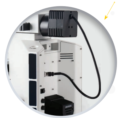
Both transmitted and reflected light options with independent light intensity control.
