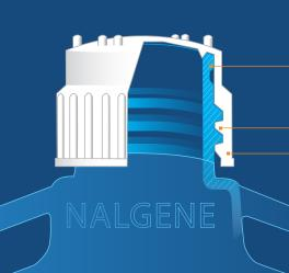
**Seal Ring** is molded inside the closure. It fits tightly against the beveled inner edge (chamfer) of the bottle neck. For dis-similar materials (e.g., HDPE carboy with PP closure) no gasket is required. For PP-to-PP sealing a gasket is added for extra security of the seal.
