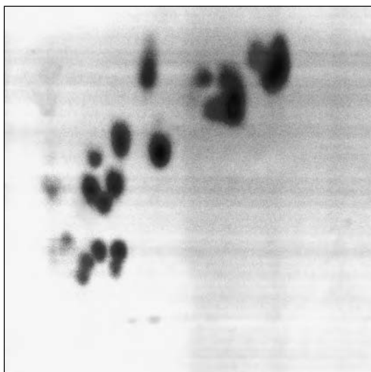
2-dimensional separation of amino acids on a HPTLC cellulose plate
