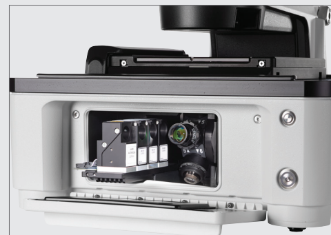
Easy access to filter/LED cubes and objectives.
