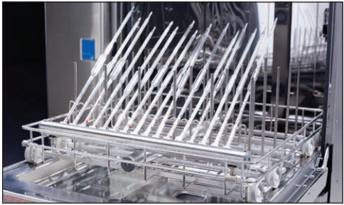
Pipets may be thoroughly washed and dried in FlaskScrubber and FlaskScrubber Vantage Series Washers. Pipet Inserts attach to the spindle rack to allow the interior of the pipets to be injected with water and detergent for washing followed by hot air for drying.
