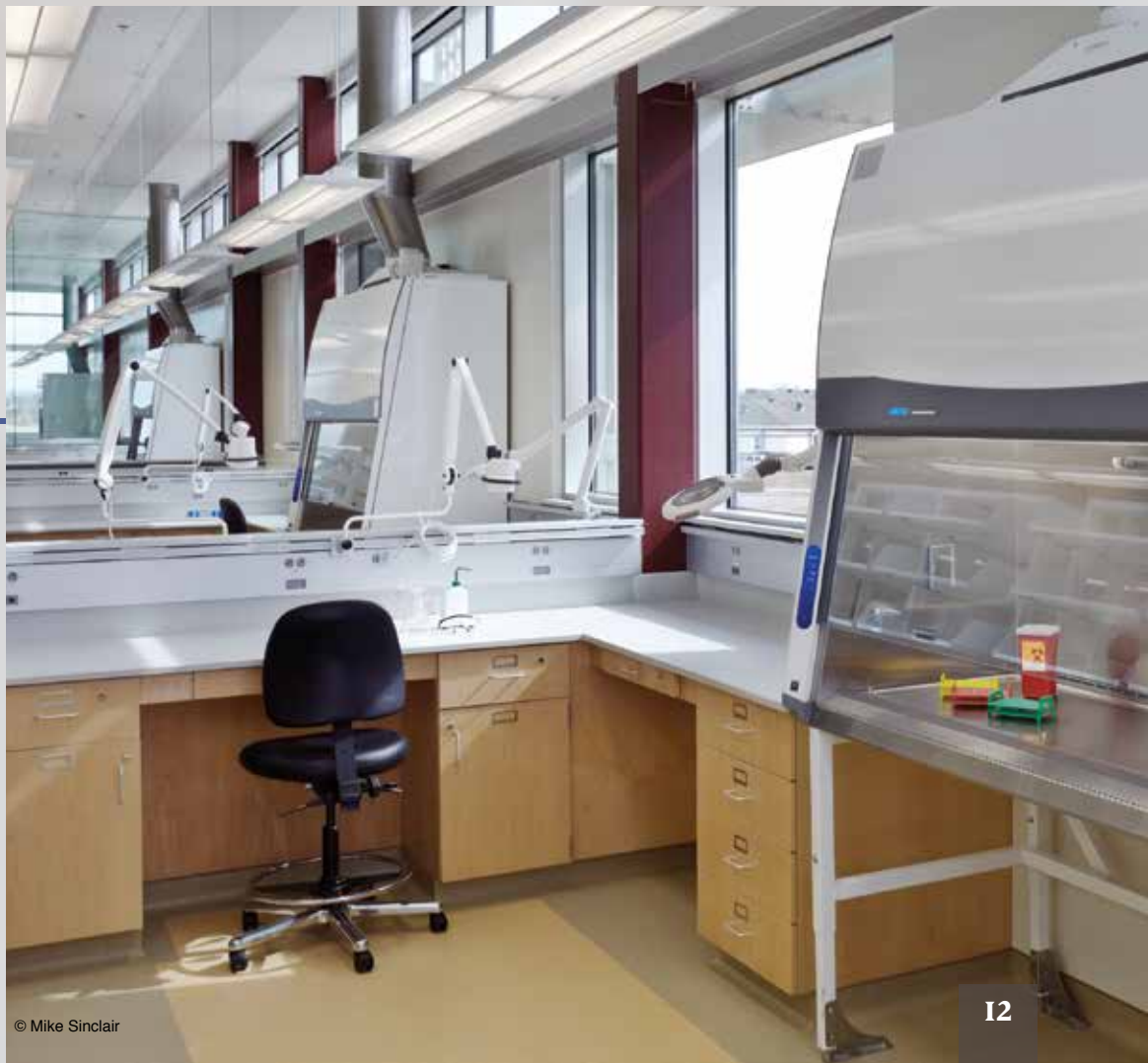
Purifier Horizontal Clean Benches produce particulate-free air in the work area to protect samples such as plant tissue from airborne contaminants.
