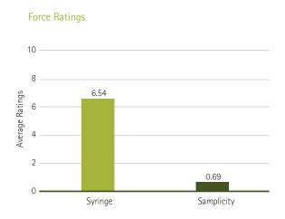
Average user ratings of manual force required and comfort levels for operating syringe filters vs. the Samplicity Filtration System show the Samplicity system requires virtually no manual force for filtration.\*
