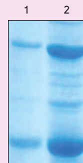
Lane 1: Brand V retentate after 5 x 60 minutes spin Lane 2: Millipore Amicon Ultra-15 filter retentate after 6 x 20 minutes spin
