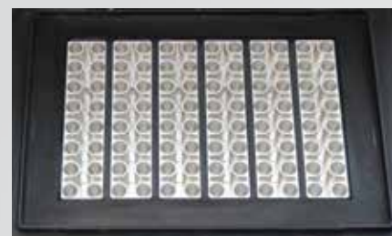
The VeriFlex Block provides independent temperature zones.
