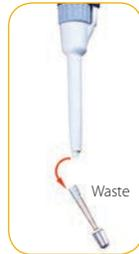
Eject to dispose of tip and FLOWMI
